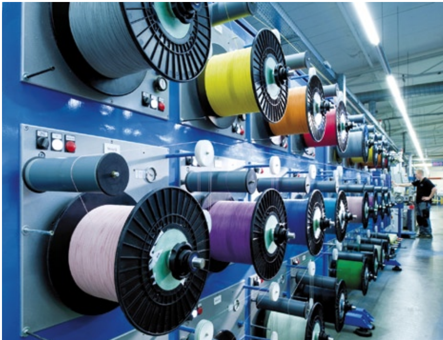
Production of fiber-optic-cables, detail of a jacketing line. (Courtesy of LEONI AG)
