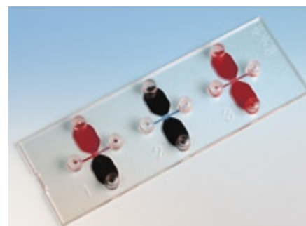
The Biophotonics Research Program helped ibidi lay the basics for their series of advanced microslides and cell chambers for live cell microscopy, including this slide for the observation of directed cell motion ("chemotaxis"). (Courtesy of ibidi)
