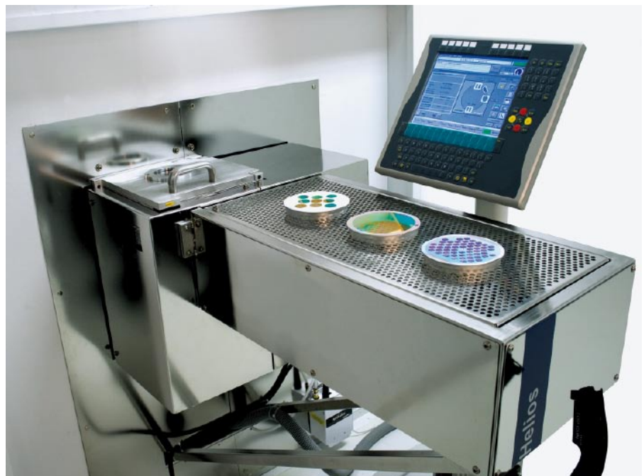
FIGURE 3: The Advanced Plasma Reactive Sputtering (APRS) Platform offers the ability to deposit hundreds of highly accurate shift-free layers per single coating run.
