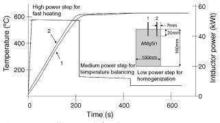
Figure 1.7 Typical heating cycle for AlMgSi1.
