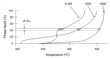
Figure 1.10 Liquid fraction as a function of temperature for various aluminium alloys [33].
