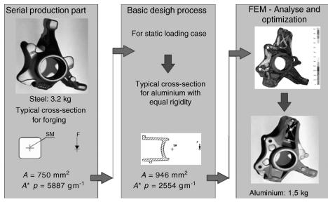
**Figure 1.12** Substituting original forged steel steering knuckle (weight 3.2 kg) by A357 semi-solid casting (weight 1.5 kg) [44].
