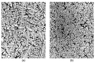
Figure 1.1 (a) Dendritic and (b) globular microstructure.
