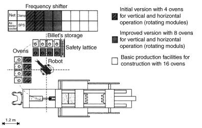
Figure 1.9 Individual coil heating system [31, 32].
