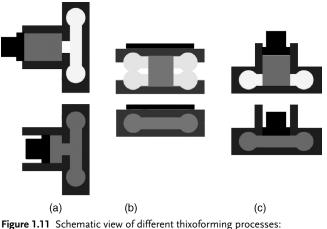
(a) thixocasting; (b) thixoforging; (c) thixo lateral extrusion.
