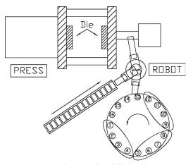
Figure 1.8 Carousel-type machine billet heating system.
