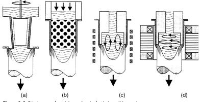
**Figure 1.6** Stirring modes: (a) mechanical stirring; (b) passive stirring; (c) electromagnetic 'vertical' stirring; (d) electromagnetic 'horizontal' stirring.
