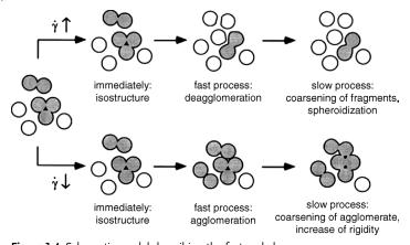
Figure 1.4 Schematic model describing the fast and slow processes in a semi-solid material's structure after up and down jumps of shear rate [16].
