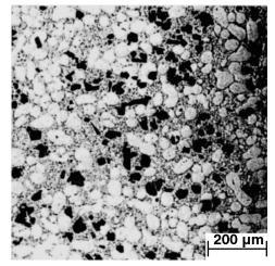
**Figure 1.13** Diesel injection pump housing semi-solid cast from A390 and microstructure with even distribution of primary silicon.
