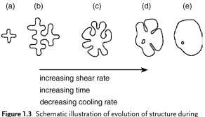
Figure 1.3 Schematic illustration of evolution of structure during solidification with vigorous agitation: (a) initial dendritic fragment; (b) dendritic growth; (c) rosette; (d) ripened rosette; (e) spheroid [15].
