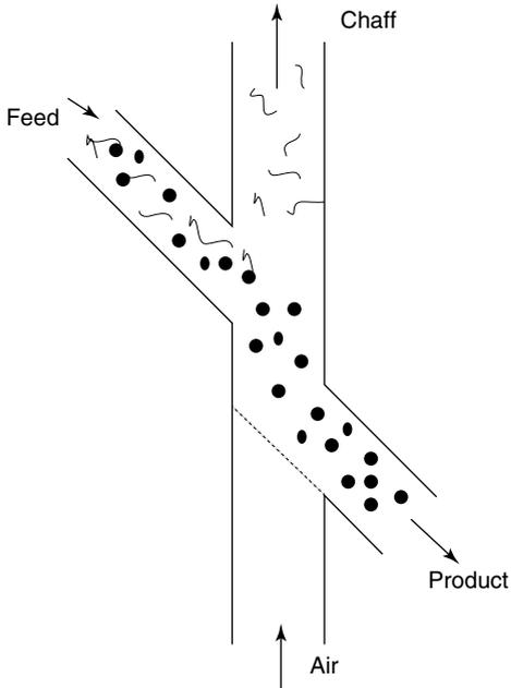
Figure 1.3 Principle of aspiration cleaning.
