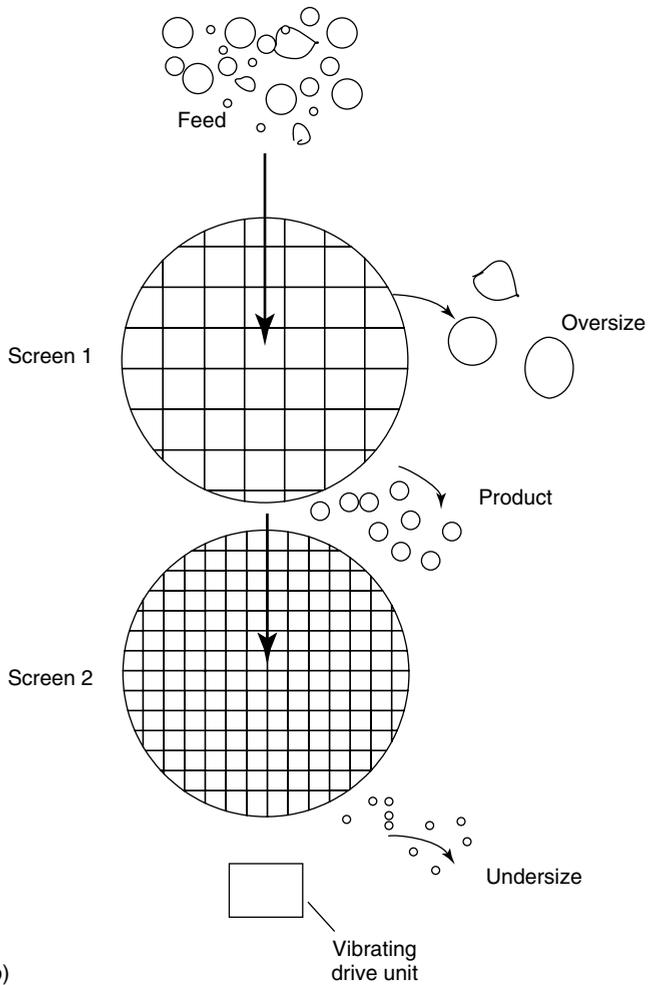
**Figure 1.2** Screen geometries: (a) rotary screen and (b) principle of flatbed screen.
