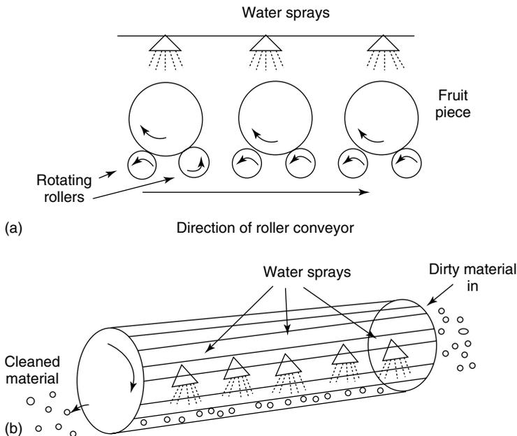
**Figure 1.5** Water spray cleaning: (a) spray belt washer and (b) drum washer.
