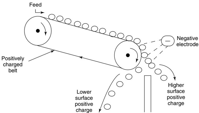
Figure 1.4 Principle of electrostatic cleaning.
