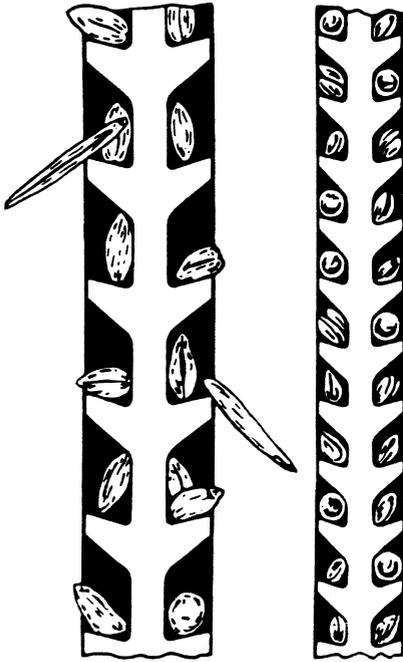
**Figure 1.8** Cross section of disk separators for cleaning cereals.
