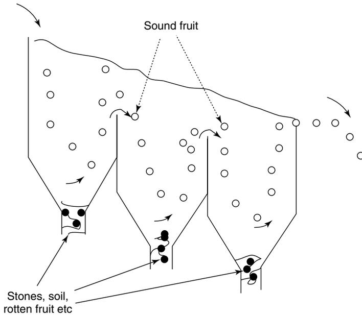
**Figure 1.6** Principle of flotation washing.
