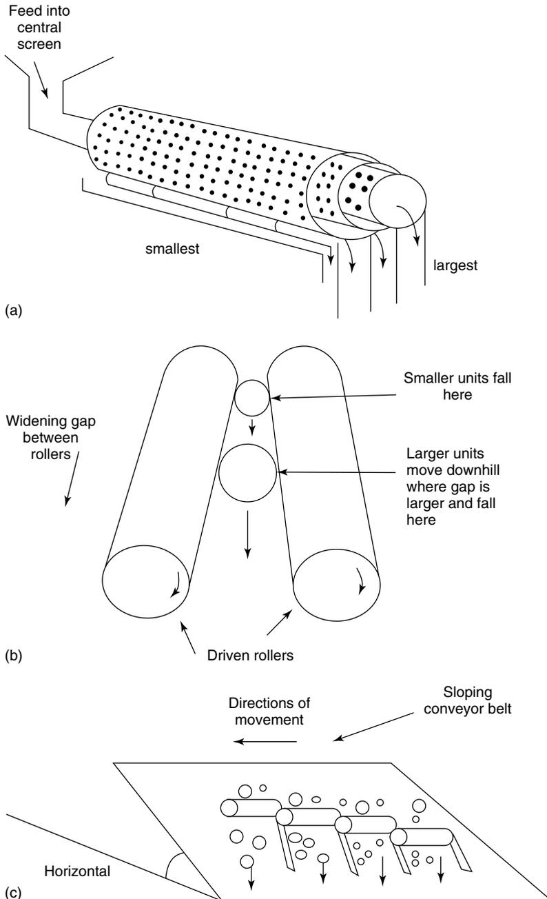
**Figure 1.7** Some geometries of size-sorting equipment: (a) concentric drum screen; (b) roller size-sorter; and (c) belt and roller sorter.
