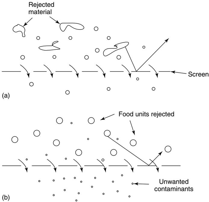
**Figure 1.1** Screening of dry particulate materials: (a) scalping and (b) de-dusting.
