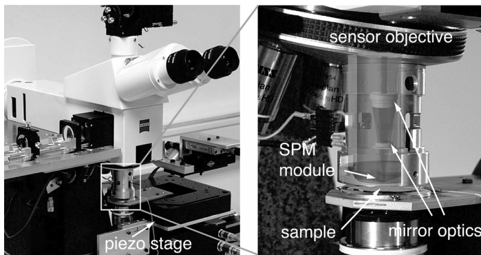
Fig. 1.2 Conventional standard microscope with screwed-in sensor objective – the version shown here allows the device to be operated as optical near-field microscope in addition to scanning force and optical microscopy. The enlarged image section in addition shows a diagrammatic representation of the beam path inside the objective.
