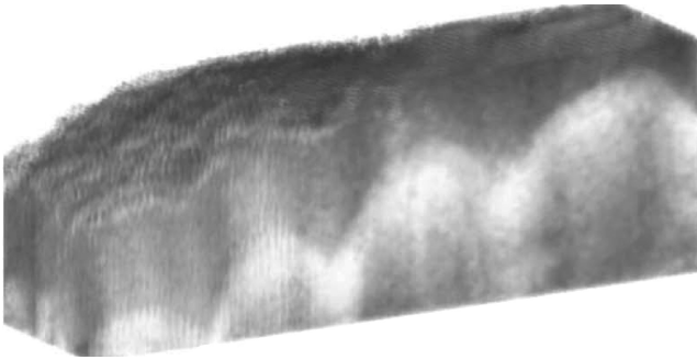
Figure 1.18 Three-dimensional skin tissue image obtained using optical coherence tomography using a quantum dot-based semiconductor optical amplifier. (Source: Krstajić et al. 2011 [44]. Reproduced with permission of IEEE Photonics Technol Lett.)
