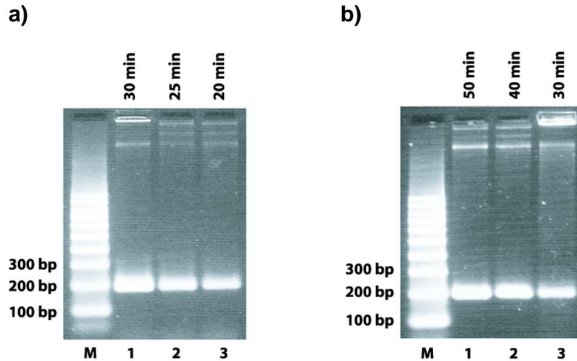
**Supplementary Figure 8.** Amplification as a function of reaction time for a 191 bp target associated with membrane channel proteins M1 and M2 of the influenza-A virus. Lane M: 100 bp marker, lanes 1-3: amplification products after various reaction times (indicated at the top of each gel image) in reactor volumes of a) 16  $\mu$ L (400  $\mu$ m dia., 69 s cycle time), and b) 10  $\mu$ L (320  $\mu$ m dia., 102 s cycle time).
