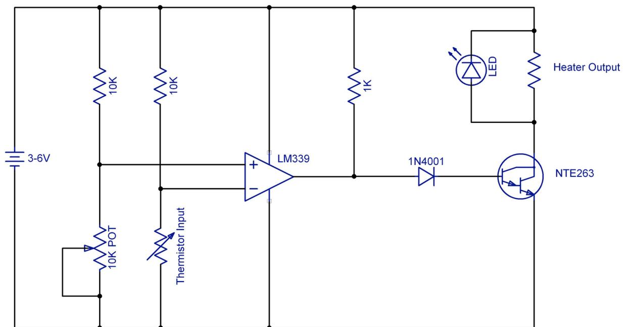
**Supplementary Figure 5.** Schematic diagram of the temperature control circuit employed in the battery powered thermocycler shown in Supplementary Figure 4c.
