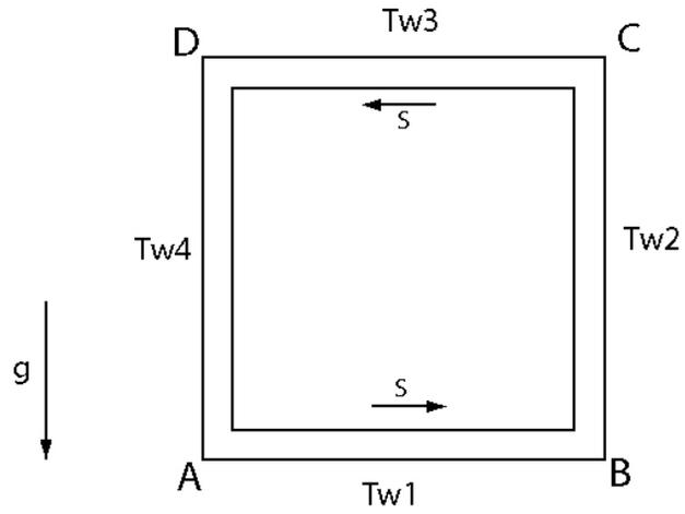
**Supplementary Figure 6.** Schematic of a square convective flow loop geometry. Point ‘A’ is the arbitrary origin and spatial coordinate  $s$  extends from ‘A’ in counterclockwise direction. The loop has a total length  $L$ , with equal segments of length  $L/4$ . Each segment is maintained at a constant wall temperature  $T_{w,i}$ .
