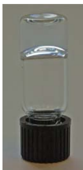
Figure S5: Gel formation in the mixture of 1 and Zn-L_2EO_4 at [1] = 7.9 g/L and pH 5.4 (with [+] = [-] = 5.8 mM, diameter of flask \sim 1 cm).
