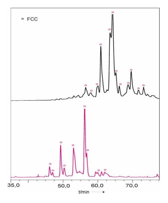
**Figure S5**. HPLC analyses of extracts of a yellow banana leaf (top) and of a yellow banana peel (bottom), with detection of luminescence at 450 nm; FCC fractions are labelled with a dot (tentative on-line identification by their UV/Vis-spectra).
