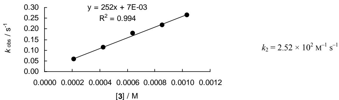
Rate constants for the reactions of 2,5-dimethylpyrrole (**3**) with (dpa)<sub>2</sub>CH<sup>+</sup>BF<sub>4</sub><sup>-</sup> (**8h**) in CH<sub>3</sub>CN (20 °C, stopped-flow,  $\lambda = 672$  nm)
