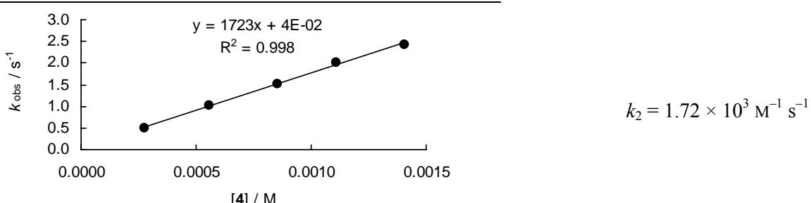
Rate constants for the reactions of 1,2,5-trimethylpyrrole (**4**) with  $(\text{dpa})_2\text{CH}^+\text{BF}_4^-$  (**8h**) in  $\text{CH}_3\text{CN}$  (20 °C, stopped-flow,  $\lambda = 672 \text{ nm}$ )
