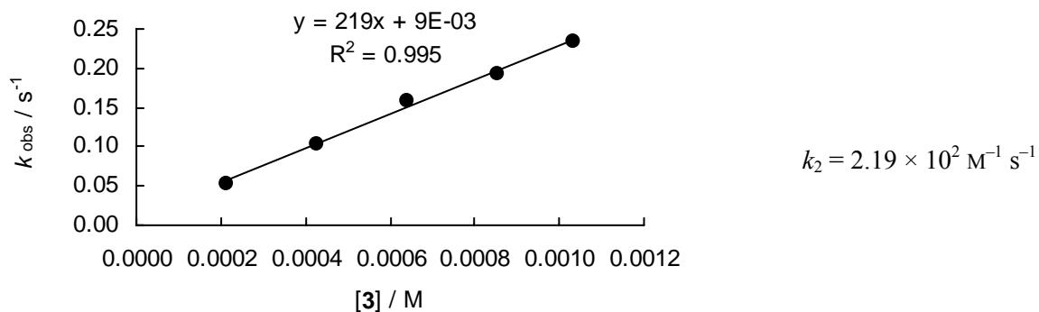
Rate constants for the reactions of 2,5-dimethylpyrrole (**3**) with (mor)<sub>2</sub>CH<sup>+</sup>BF<sub>4</sub><sup>-</sup> (**8g**) in CH<sub>3</sub>CN (20 °C, stopped-flow,  $\lambda = 620$  nm)
