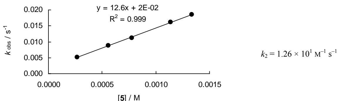
Rate constants for the reactions of 2,4-dimethylpyrrole (**5**) with  $(\text{ind})_2\text{CH}^+\text{BF}_4^-$  (**8c**) in  $\text{CH}_3\text{CN}$  (20 °C, J&M,  $\lambda = 625 \text{ nm}$ )
