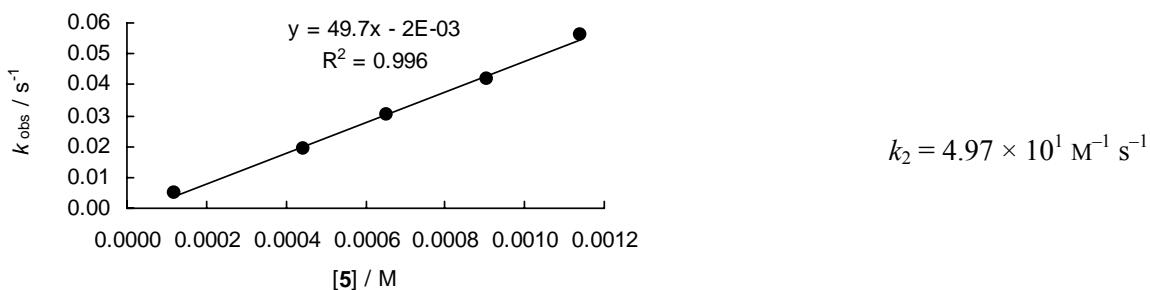
Rate constants for the reactions of 2,4-dimethylpyrrole (**5**) with  $(\text{pyr})_2\text{CH}^+\text{BF}_4^-$  (**8d**) in  $\text{CH}_3\text{CN}$  (20 °C, stopped-flow,  $\lambda = 620 \text{ nm}$ )
