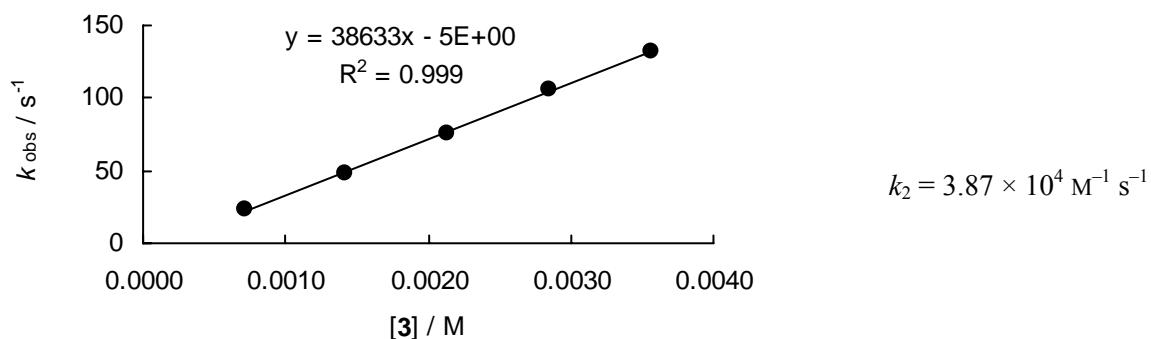
Rate constants for the reactions of 2,5-dimethylpyrrole (**3**) with  $(\text{mfa})_2\text{CH}^+\text{BF}_4^-$  (**8i**) in  $\text{CH}_3\text{CN}$  (20 °C, stopped-flow,  $\lambda = 593 \text{ nm}$ )
