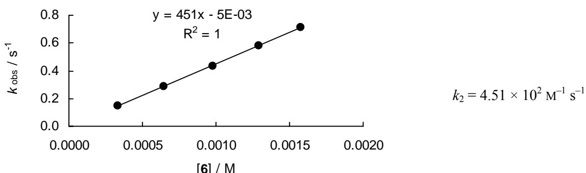
Rate constants for the reactions of 3-ethyl-2,4-dimethylpyrrole (**6**) with (pyr)<sub>2</sub>CH<sup>+</sup>BF<sub>4</sub><sup>-</sup> (**8d**) in CH<sub>3</sub>CN (20 °C, stopped-flow,  $\lambda = 620$  nm)
