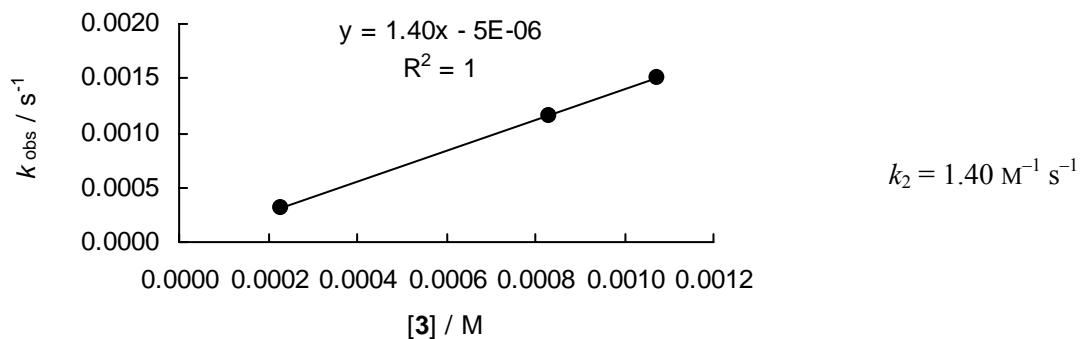
Rate constants for the reactions of 2,5-dimethylpyrrole (**3**) with  $(\text{mpa})_2\text{CH}^+\text{BF}_4^-$  (**8f**) in  $\text{CH}_3\text{CN}$  ( $20^\circ\text{C}$ , stopped-flow,  $\lambda = 622 \text{ nm}$ )
