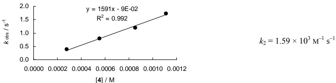
Rate constants for the reactions of 1,2,5-trimethylpyrrole (**4**) with (mpa)<sub>2</sub>CH<sup>+</sup>BF<sub>4</sub><sup>-</sup> (**8f**) in CH<sub>2</sub>Cl<sub>2</sub> in presence of *N*-methyl morpholine (NMM) (20 °C, J&M,  $\lambda = 622$  nm)
