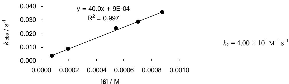
Rate constants for the reactions of 3-ethyl-2,4-dimethylpyrrole (**6**) with  $(\text{ind})_2\text{CH}^+\text{BF}_4^-$  (**8c**) in  $\text{CH}_3\text{CN}$  ( $20^\circ\text{C}$ , stopped-flow,  $\lambda = 625 \text{ nm}$ )
