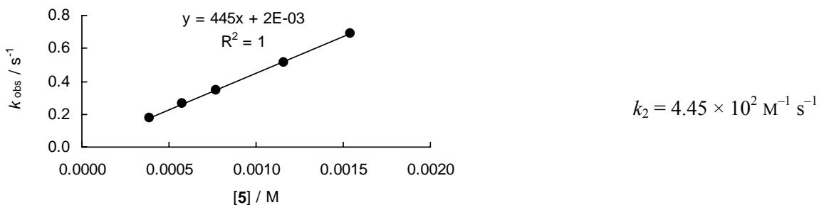
Rate constants for the reactions of 2,4-dimethylpyrrole (**5**) with  $(\text{mpa})_2\text{CH}^+\text{BF}_4^-$  (**8f**) in  $\text{CH}_3\text{CN}$  (20 °C, stopped-flow,  $\lambda = 622 \text{ nm}$ )
