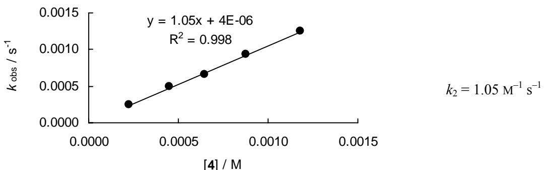
Rate constants for the reactions of 1,2,5-trimethylpyrrole (**4**) with (pyr)<sub>2</sub>CH<sup>+</sup>BF<sub>4</sub><sup>-</sup> (**8d**) in CH<sub>3</sub>CN (20 °C, J&M,  $\lambda = 620$  nm)
