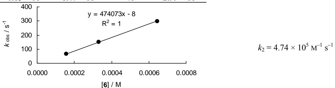
Rate constants for the reactions of 3-ethyl-2,4-dimethylpyrrole (**6**) with (mor)<sub>2</sub>CH<sup>+</sup>BF<sub>4</sub><sup>-</sup> (**8g**) in CH<sub>3</sub>CN (20 °C, stopped-flow,  $\lambda = 620$  nm)
