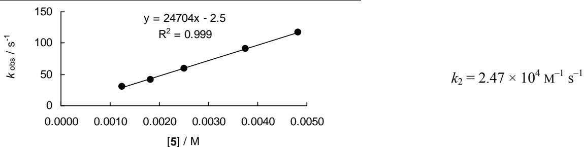
Rate constants for the reactions of 2,4-dimethylpyrrole (**5**) with (mor)<sub>2</sub>CH<sup>+</sup>BF<sub>4</sub><sup>-</sup> (**8g**) in CH<sub>3</sub>CN (20 °C, stopped-flow,  $\lambda = 620$  nm)
