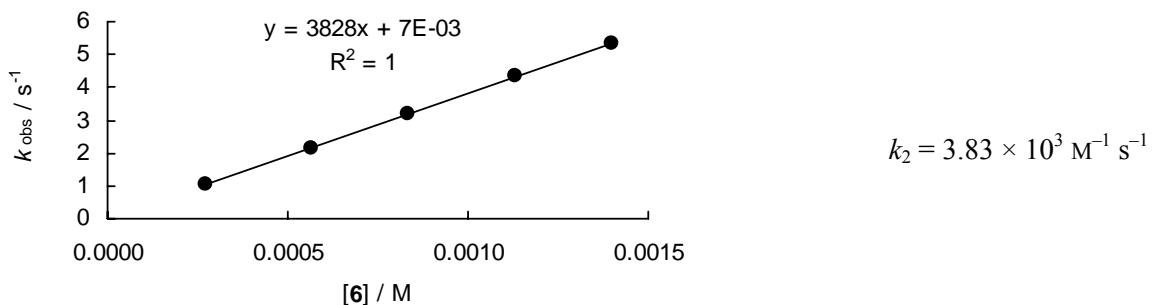
Rate constants for the reactions of 3-ethyl-2,4-dimethylpyrrole (**6**) with (mpa)<sub>2</sub>CH<sup>+</sup>BF<sub>4</sub><sup>-</sup> (**8f**) in CH<sub>3</sub>CN (20 °C, stopped-flow,  $\lambda = 625$  nm)
