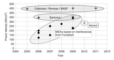
**Figure 1.3** Power densities of MEAs manufactured by different developers [56–71] for comparable operating conditions. Temperature,  $160^{\circ}$ C; fuel, pure hydrogen, pressure; 1 bar; cell voltage, 0.5 V.
