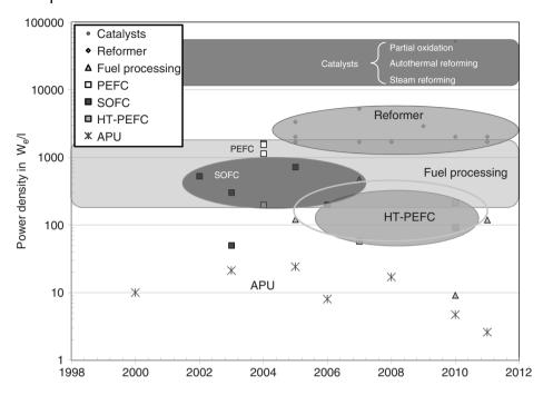
Figure 1.8 Power densities achieved for catalysts, reformers, fuel processing systems, fuel-cell stacks, and APUs.
