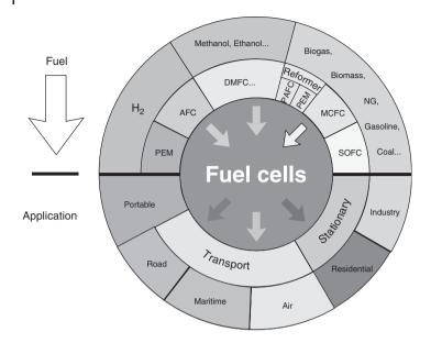
Figure 1.1 Fuel-cell technologies, possible fuels, and applications [1].
