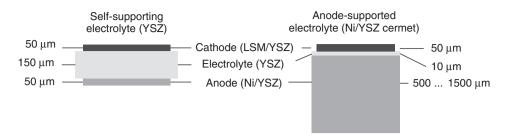
Figure 1.2 Anode substrate (right) in comparison with electrolyte substrate (left).
