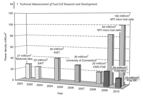
**Figure 1.4** Development of the power density of passive DMFC systems at room temperature  $(20-30^{\circ}C)$ .
