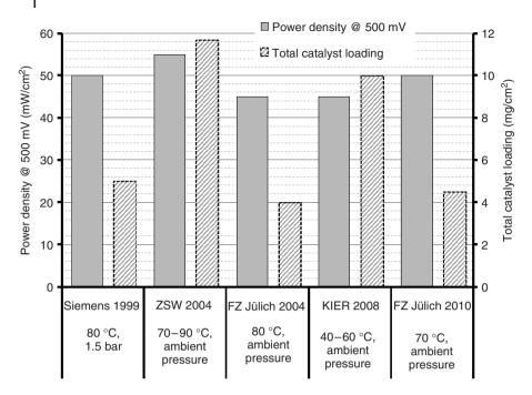
**Figure 1.5** Specific power densities of membrane electrode assemblies in DMFC stacks in the power class >100 W.
