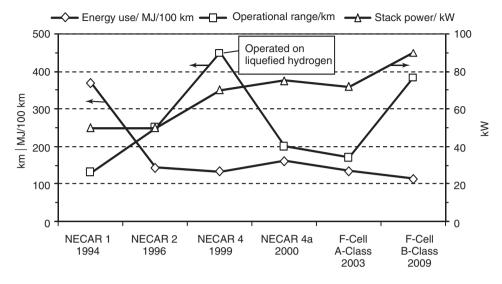
Figure 1.6 Development of range, stack performance, and energy demand of FCHVs.
